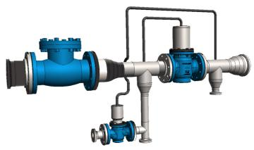
With the HYDROMINE<sup>™</sup> LFC\_3B flow control systems, the water will be returned to the mining production pipe line and while there is a flow demand, flow will remain constant and the coils will operate at their designed flow rate, making this system very efficient.
